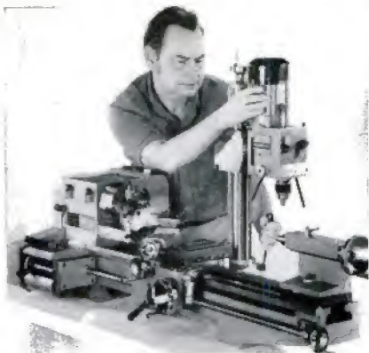
FOR LATHEWORK , machine's vertical head can be swung out of the way. The column rotates full 360°
